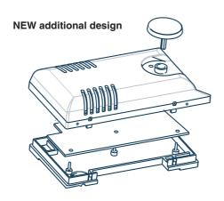
Enclosure with knob, for wall mounting, suitable for room thermostats etc. A knob fits among others trimmer PCH 215/30 and another knob for encoder can be used. See www.Bernic.dk. Standard colour is white/black but other colours can be supplied upon request. PCB and packing are available. Base part available with cold pressfixing taps or for selftapping screws to fix the PCB.
