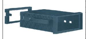
This enclosure can easily be assembled without the use of fixing screws. The PCB is inserted from the rear side of the enclosure using the internal PCB guides and it is fixed by the rear frame with a snap-lock mechanism. Either the front or the rear panels can be inserted into the enclosure by a snap-lock mechanism. Lengths (L) different from the standard ones are available upon request.
